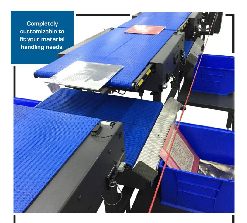
Our Transpositor provides right-angle product transfers and allows product lanes or patterns to be built across the width of receiving conveyors. The transfer function uses our sprocket-driven Microspan Chain.
