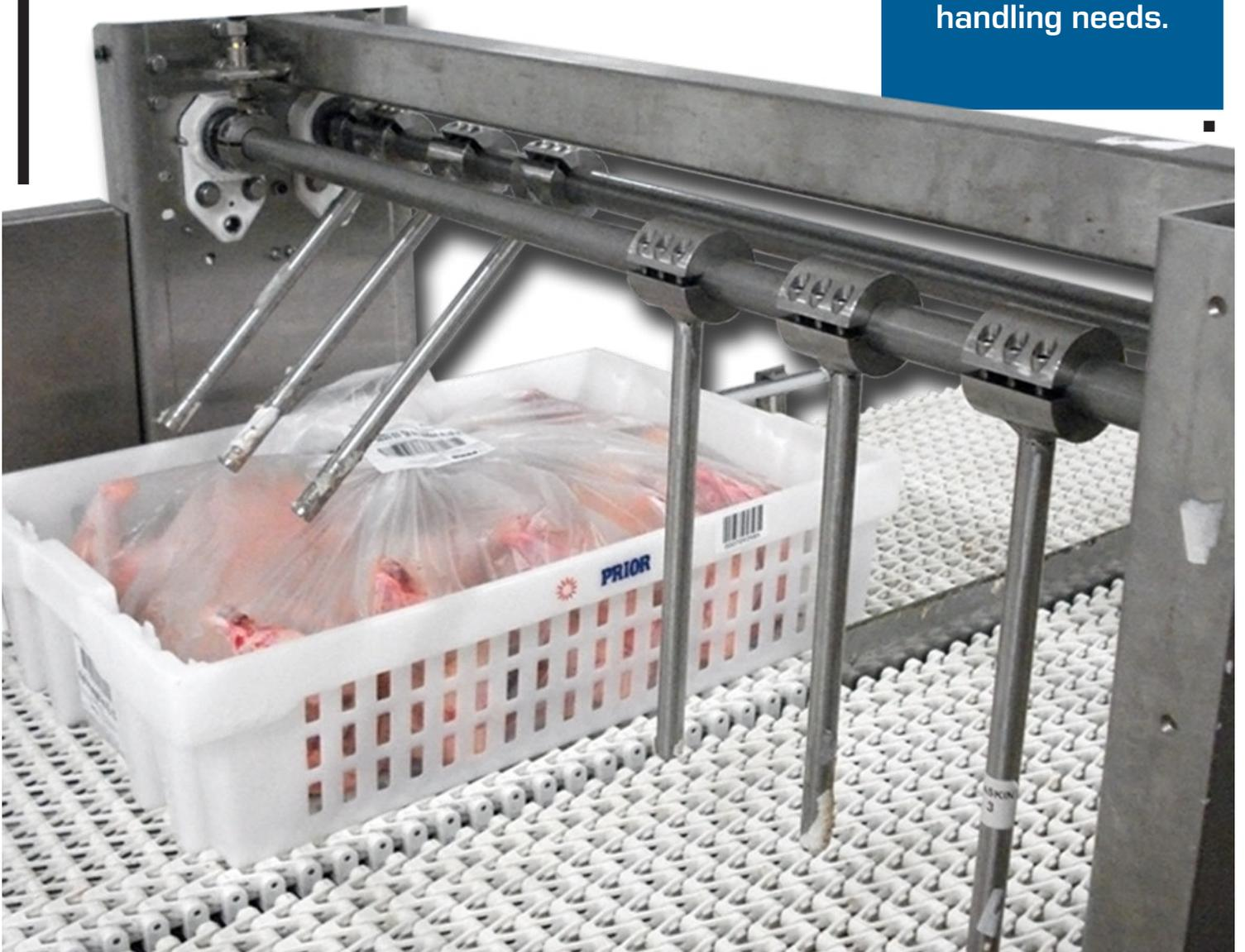
The Traffic Cop merges two lanes of product into a single lane of output regardless of the varying sizes of your product. It operates without sensing devices, I/O components or powered automation.
