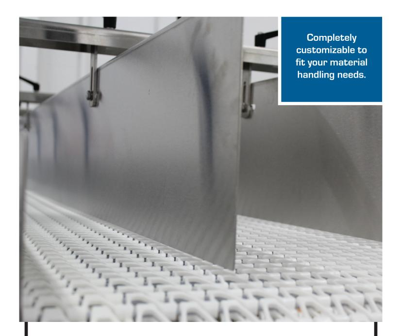
Side Walls can be customized to fit your specific applications and are an effective way to guard against the moving sides of the conveyor chain. Based on your needs, sidewalls are available in stainless steel, UHMW, and Lexan.
